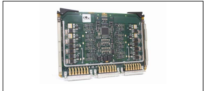
Figure 2. DDC RP-26200 16-Channel Solid State Power Controller Board.
